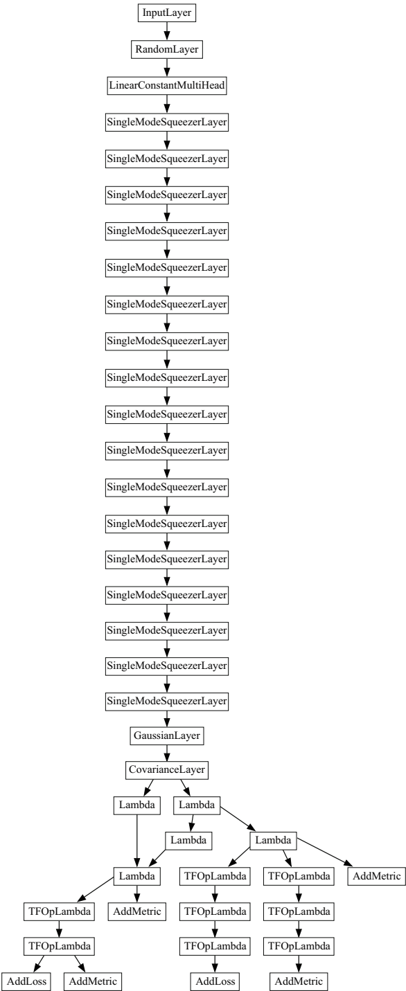
Fig. 13.2 Model for the BSVA with various squeezing layers and the measurement layers
